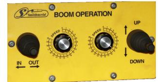
Non-latching, joystick & speed control, for super fine weld head adjustments. Located where you need it.
